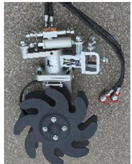
2 blade Rotary hoe with hyd. offset control
