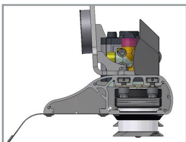
CROSS SECTION OF CUTTER BAR
