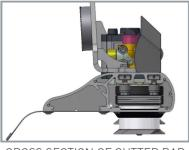
CROSS SECTION OF CUTTER BAR
