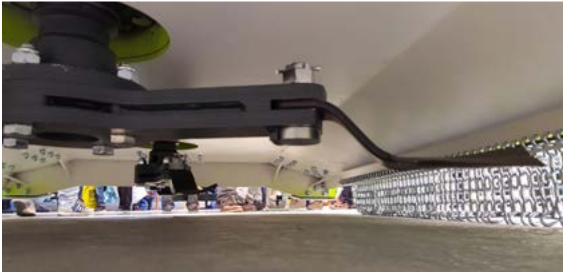
HD flail and carrier plate system
