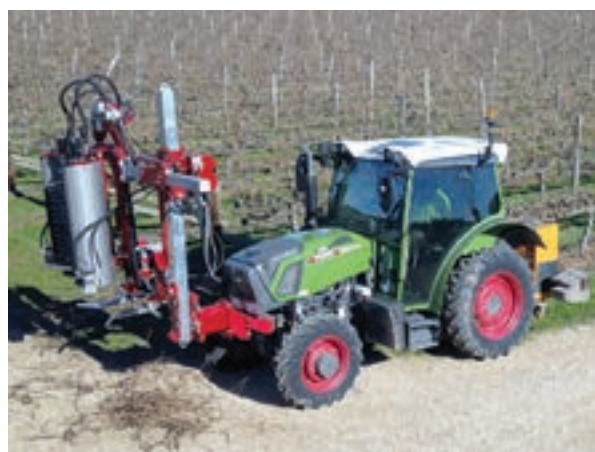
ERO VSL HD pruner with high-speed saws on XHD mast
